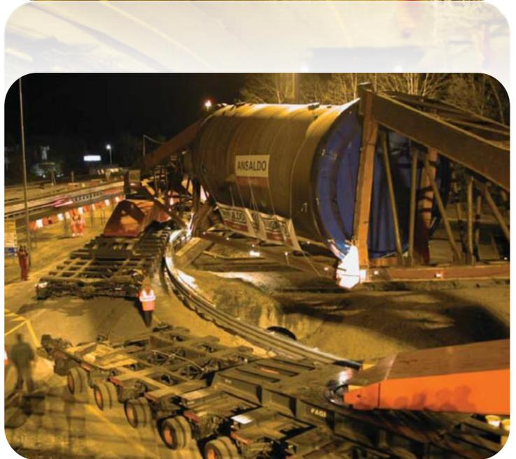
The barge moved the load to the docking facility designed by Fagioli to offload the steam generators using the tide cycles.
