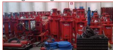
Strand jacks load test are executed up to 120% load capacity before shipment to site. For further details on strand jacking system, please refer to "FAGIOLI TECHNICAL DATA STRAND JACKING SYSTEM" document.
