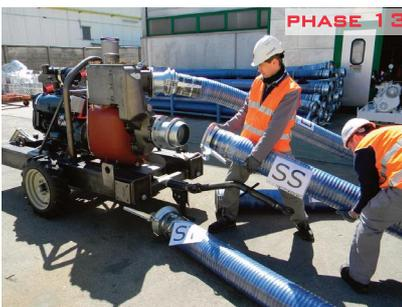
**PHASE 11:** A ballasting operator supports the hose while the second Ballasting Operator release the main quick coupling.
