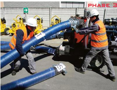
**PHASE 4:** Release the secondary quick coupling.
