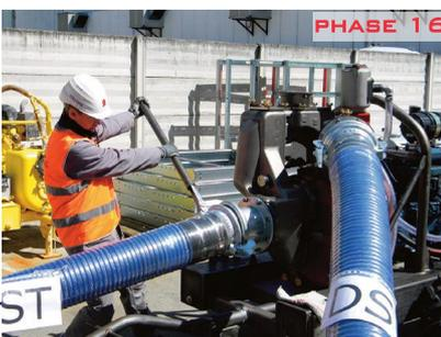
**PHASE 15:**The secondary quick coupling is locked on the hose connection.
