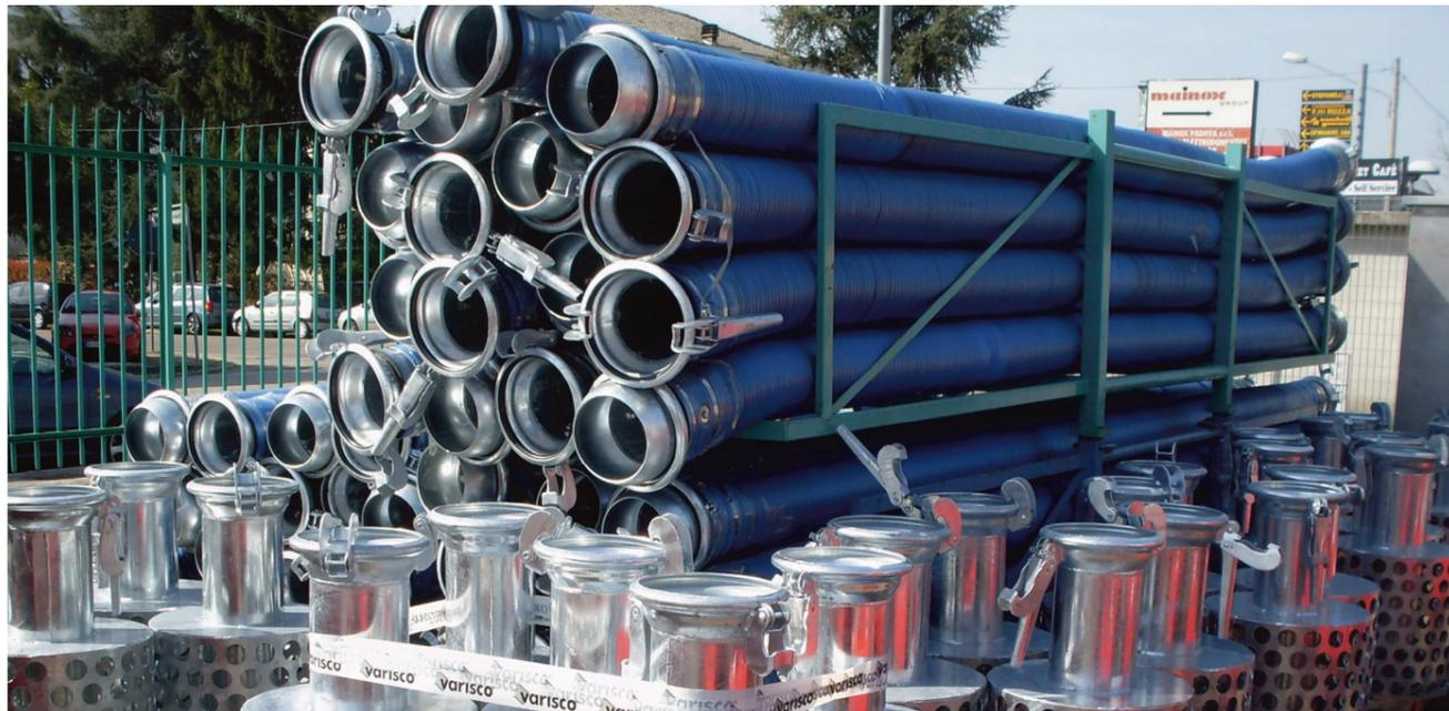
The pipe lines of the system are composed by hoses with a diameter of 8" equivalent to 200mm. This size allows the reduction and optimization of the loss of pressure during pumping. In case of emergency the pump flow can require to be reversed. Fagioli always arrange contingency hoses close to the pumps in order to be quickly connected to the pumps reversing the flow if required.
