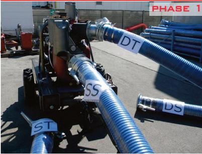
**PHASE 1:** Switch-off the engine pump.
