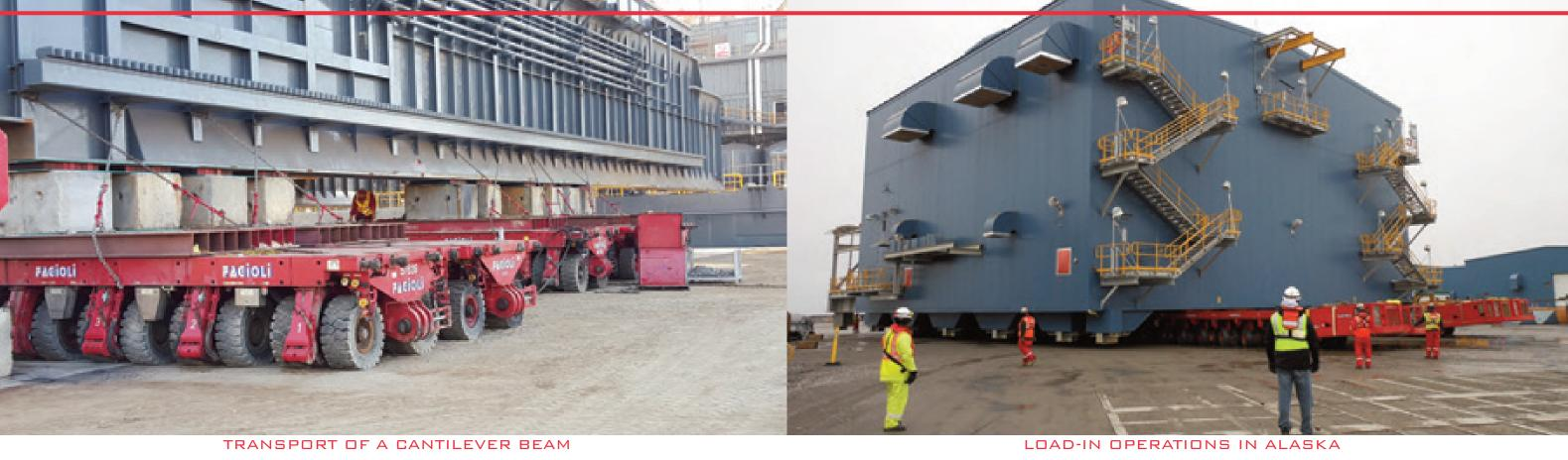
Fagioli Inc. USA was awarded the SPMT transport operations of a 1905 ton cantilever structure and a drill-floor package in Texas. Dimensions of the cantilever were:  $42 \text{ m} \times 21.5 \text{ m} \times 75 \text{ m}$ . Fagioli provided No. 88 lines of SPMTs and No. 5 power pack units (1 spare included). First Fagioli performed the weighing of the heavy items by means of SPMTs, then after
