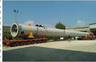
like a sword of Damocles. Picture top left shows the transport and loading activity of a heavy item destined to North Europe. Picture in the middle refers to the transport and loading operations at Venice port of a 41 m long vessel column executed with a convoy composed by 7 + 7 axle lines trailers with drawbar connecting beam, destined to United States.
