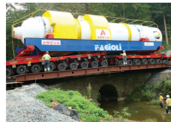
USA: Challenging passage onto a bridge with SPMTs onto a Fagioli overbridge for the TMI project.
