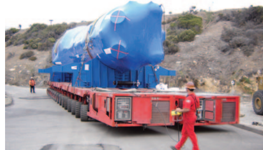
USA: Transport of No.4 x 327 ton each Steam Generators from Spain to USA
