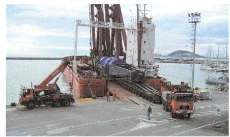
The 284 tonne gas turbine positioned onto Fagioli SPMTs in Civitavecchia was transported into a storage area in order to be transhipped onto 15+15 axles lines fitted with girder beams.
