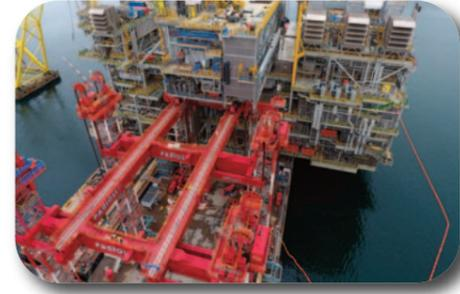
Alternative lifting equipment used in Heavy Haulage and Lifting operations. In addition to the equipment described above, Fagioli has in its fleet other assets as hydraulic lifting frames of variable height (gantry systems), modular towers, hydraulic cylinders with a set of steel cables, used to pull and lift (strand jacks) and skid shoes (above 1,000 ton capacity each) for the lifting, skidding and installation of heavy items.
