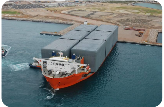
Below: Arrival of tanks at Algeciras construction site
